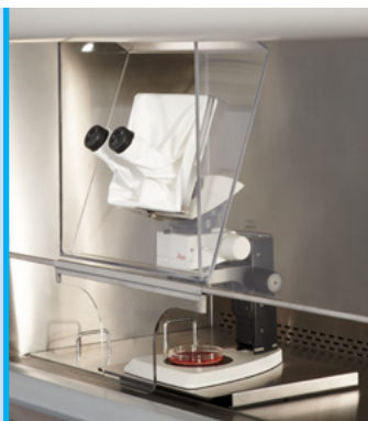
This LabGuard BSC was fitted with a microscope viewing window to accommodate workflow specializing in human cell tissue research.
