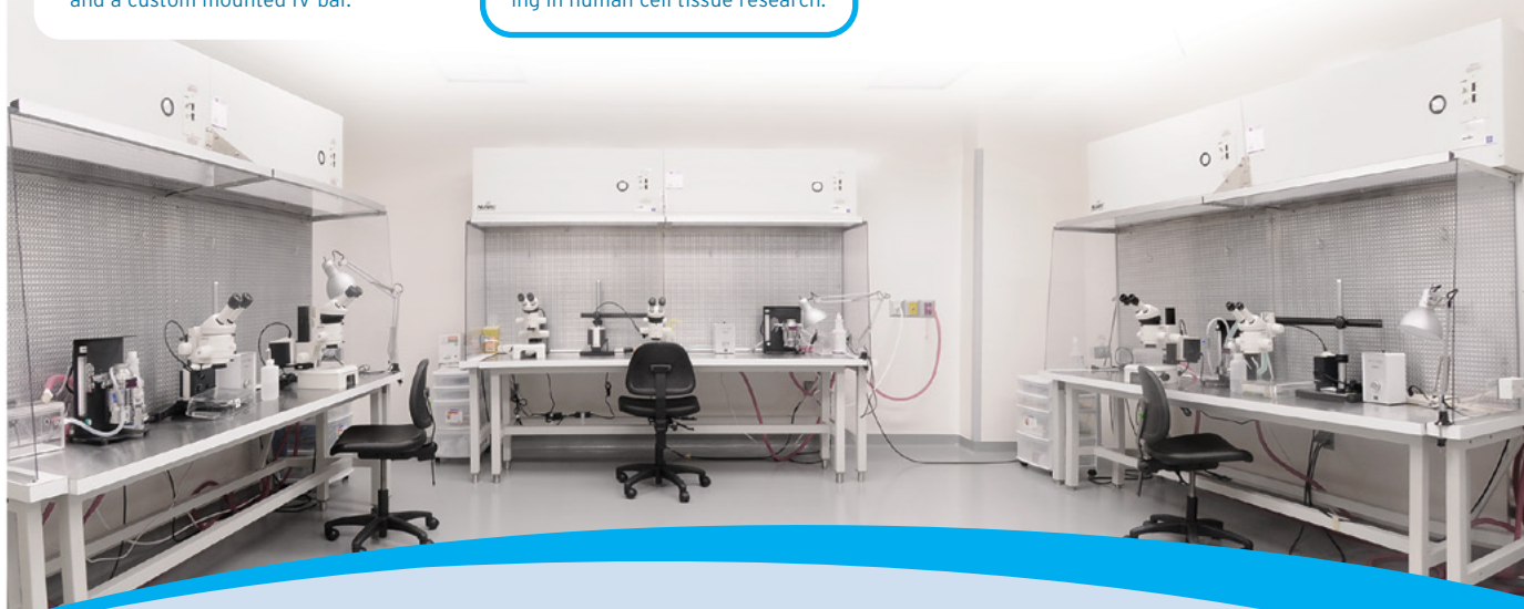
This Class I BSC was created at a nominal width of 8' [2.4 m], with clear polypropylene sidewalls, and a custom mounted IV bar.
