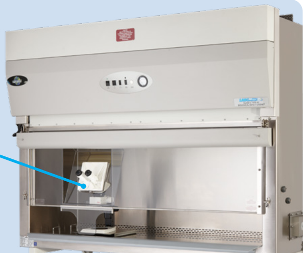
This LabGuard BSC was fitted with a microscope viewing window to accommodate workflow specializing in human cell tissue research.
