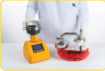
1. Remove the protective cover head from AIRBIO
