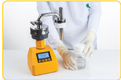
4. Connect the bottle with the collection liquid
