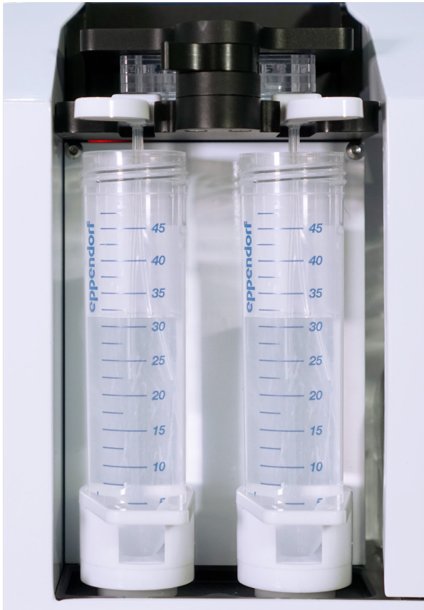
two 50 ml centrifuge tubes hold sample/buffer
