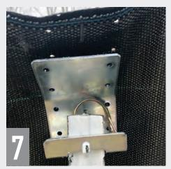
Fold top edge of fabric over bracket, aligning prepunched holes in fabric with the top two holes in the bracket. (The bottom six holes are unused.)
