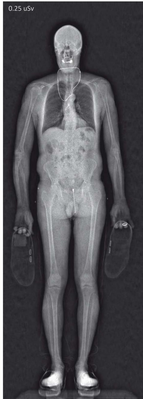
A typical image from Intercept on the lowest setting, 0.25 uSv. Items: teeth fillings, neck chain, object in shoe heel, ring and zipper. Intercept can operate at up to 200 uRem for even better image quality.
