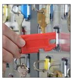
All keys secured within a KeyWatcher system are locked to a Smart Key device with built-in memory chip. Any time a Smart Key is inserted into or removed from a KeyWatcher key slot, the system stores data on time, user and more.
