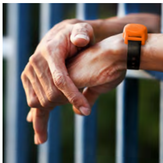
Detainee tag with heart rate monitoring
