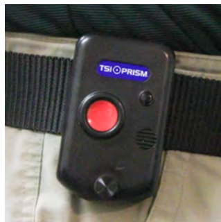
Officer tag with man down and duress functions
