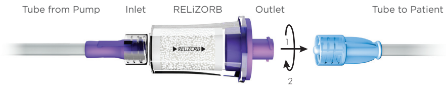
FIGURE 2: Connecting RELiZORB outlet to inlet fitting of patient extension set or enteral feeding tube that connects to patient.
