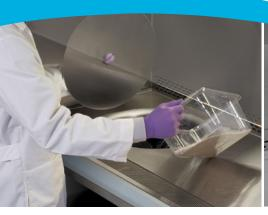
An optional waste bin can be installed into the work surface for safe and convenient disposal.
