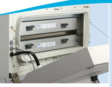
Access filters and the blower motor from the front of the cabinet with the easy removal of safety panel.
