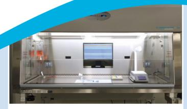
The NU-543 optimized for IV and drug compounding workflow featuring a back wall monitor viewing window, IV bar, and additional GFCI outlets.
