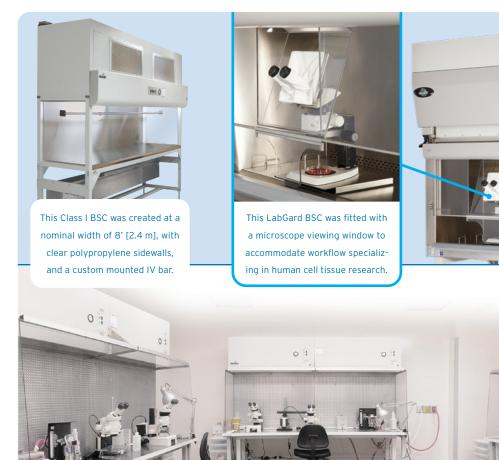
A custom model NU-240 was designed to offer a broader and taller work zone to accommodate a single workflow process involving microscopes. A customized isolation table was added to eliminate vibration in the work surface. The extended work surface allows a technician to perform several protocols without having to leave the work zone.
