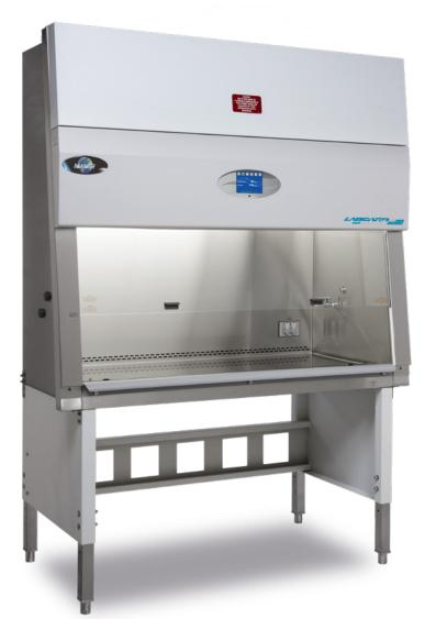
The LabGard<sup>®</sup> ES (Energy Saver) AIR Limited Model NU-545 Class II, Type A2 Biosafety Cabinet is a bench/table top model with available base stand options. The Energy Saver DC ECM motor is controlled to airflow set points via the TouchLink<sup>™</sup> central control system. The touchscreen control system utilizes two dual digital thermistor airflow sensors that provide automatic compensation for both filter loading and line voltage variances to maintain constant air volume control.
