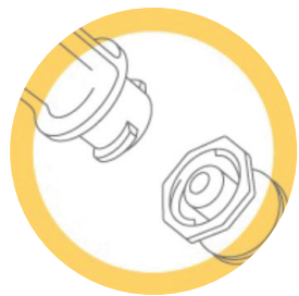
Feeding Tube (Final) Changing from male – the stepped or Christmas tree connector – to the new ENFit female connector. The feeding tube port for the administration set will change from female to male.
