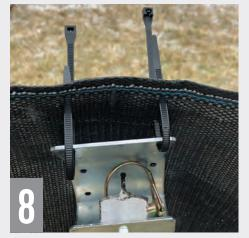
Feed two 75# zip ties through the fabric, into the bracket and back through the fabric.
