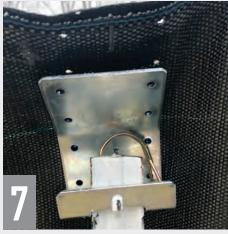
Fold top edge of fabric over bracket, aligning prepunched holes in fabric with the top two holes in the bracket. (The bottom six holes are unused.)
