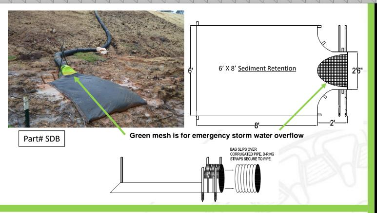
Designed to retain sediment from a 12" diameter temporary slope drain pipe. An emergency overflow has been provided in the top portion of the bag allowing excess stormwater to be released during heavy rain events and reducing the potential for separation of the slope drain pipe sections.
