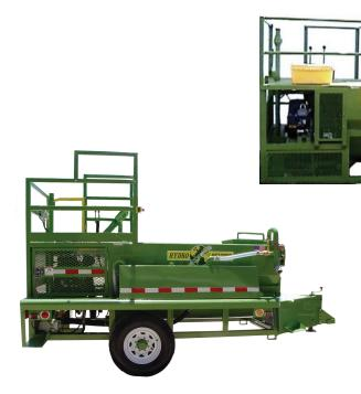
With **Bowie's Lancer 600**, you can apply your product either from the working platform using the discharge cannon or from the ground using a hose. You can cover more area with less labor. This unit uses one elecric clutch to operate the full size agitator and another to operate the pump. It is available as either a skid or trailer mounted unit. Whatever your application needs are, you can rely upon Bowie's "Built Strong....Built to Last" equipment.
