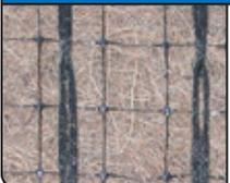
Created with three UV-stabilized nets, the three dimensional ECC-3 will provide protection through all phases of vegetation growth. The layer of coconut fiber is slow to degrade and helps with the germination. This is an excellent choice for high-flow areas and steep embankments where a permanent solution is needed.
