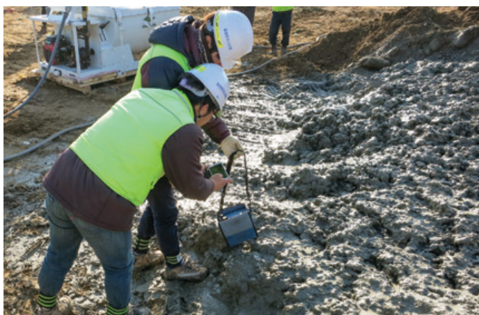
Interscan Device – Testing Odor-Shell® on freshly dumped biosolids.
