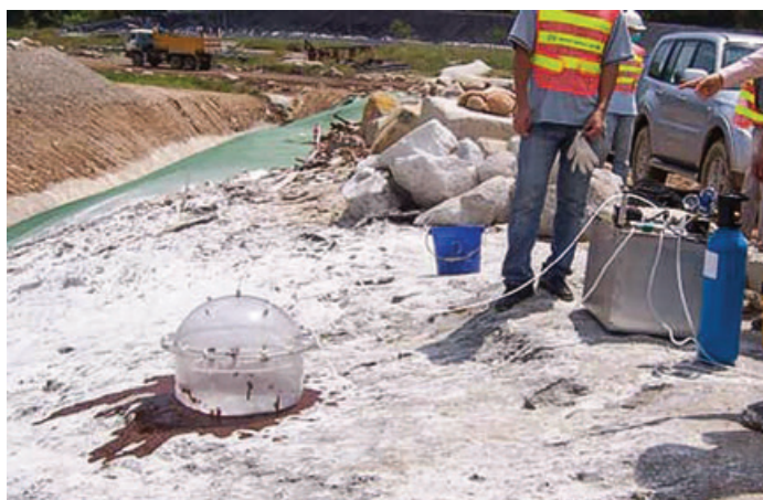
Flux Chamber – Testing Posi-Shell® for gas emissions. Dark area is wet Posi-Shell® used to seal device.
