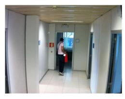
suffered from distortion created by the camera lens. Using Amped FIVE they can apply the undistort filter to correct this before attempting to analyze the suspects height.
