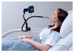
The Display Module can be mounted in the bed side rail (pictured above), or the entire system can be mounted to an IV pole for easy portability from room to room.
