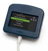
The Display Module mounts within view of the patient and provides access to nurse call, TV controls, and room controls.
