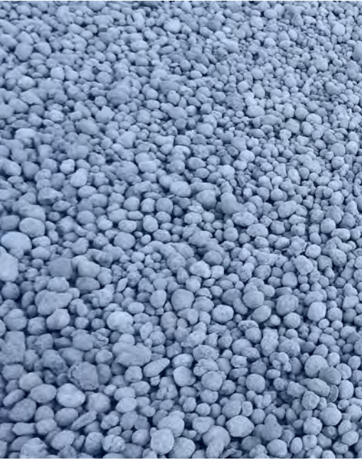
Accelerated carbonation technology (ACT) uses carbon gas to treat thermal wastes. The result is the production of stable carbonates that are blended with binders and fillers then pelletized to form artificial limestone, such as this product from Carbon 8 (Image courtesy of Carbon 8).
