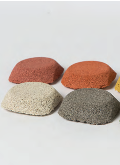
Solidia technologies produces carbon cement and cures concrete with CO 2 instead of water resulting in up to a seventy percent reduction in the carbon footprint of concrete products (Image courtesy of Solidia Technologies)
