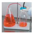
While holding the VacuCap device securely on the filtrate container, start the vacuum. The VacuCap device will seal securely to the container top and fluid will be drawn.
