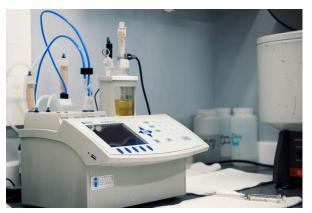
port Biodiesel used the titrator to measure the amount of moisture in the incoming cooking oil and in the finished biodiesel product. The goal in biodiesel production is to have the lowest moisture content possible in the final product. If they notice the moisture content is rising, they can proactively adjust their process and ensure a consistent result. Without a
