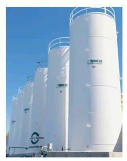
Biodiesel is produced by a process called transesterification, where fats and oils are converted into biodiesel and glycerin (as a co-product). Specifically, at Newport Biodiesel, they prepare used cooking oil for biodiesel production by removing solids and water through a mechanical operation. The oil then goes through a light chemical process involving methanol and a catalyst to emerge with biodiesel.
