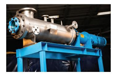
This film is constantly renewed, as the concentrated material is displaced towards the bottom discharge nozzle, by the incoming feed. As the residence time is generally measured in seconds, the degradation of heat sensitive materials is minimized.
