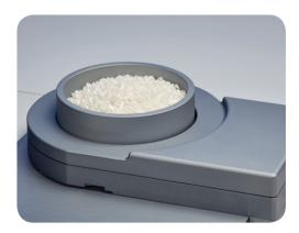
Integrating Sphere for measuring solids and semi-solids in diffuse reflection. An optional sample rotator assures a high reproducibility for heterogeneous samples.
