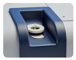
Sample Compartment, with sample heater and automated background capability, allows easy measurements of liquids in cuvettes or disposable vials.
