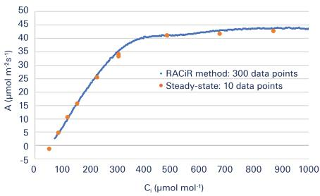
Figure 1. Comparison of a steady-state response curve (orange) and the RACiR Method (blue) on a single sunflower leaf (*Helianthus spp.*). The steady-state curve took 25 minutes, while the RACiR Method took 10 minutes at a ramp rate of 100 µmol mol<sup>-1</sup>. In ideal conditions, a RACiR curve for parameter estimation can take as little as 5 minutes.
