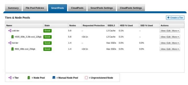
5. Edit the default file pool policy to change the storage target to *hot-tier*. This will ensure that all files are placed on the F800 nodes unless another file pool policy applies that overrides the storage target.
