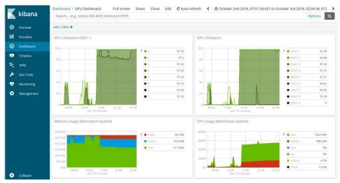
Figure 12: A custom Kibana dashboard showing GPU, CPU, and memory utilization. Data is collected by Metricbeat and NVIDIA GPU Beat.
