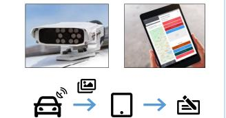
Once scanned, the CIPS system will transmit any found violation, with photos, to a mobile tablet carried by a Parking Enforcement Officer (PEO). The PEO then issues tickets only to vehicles that are identified with violations.
