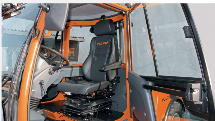
Air-suspension seat with seat heating and armrest
