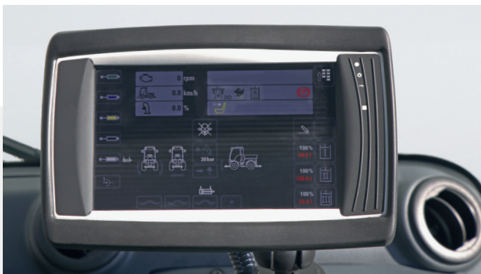
Touch display for operating all hydraulic functions
