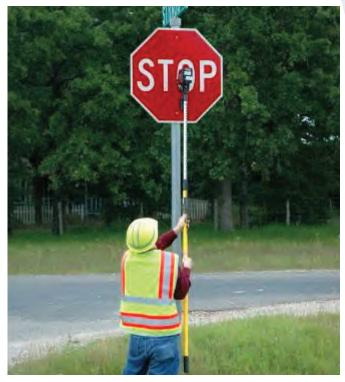
A reflectometer is used to measure the retroreflectivity of a Minnesota stop sign.
