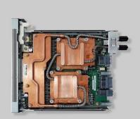
Stäubli's CGD quick release metal couplings provide a flush face, no leak solution at the point of connection and disconnection, guaranteeing the integrity of the cooling circuit. The capacity for high flow volume, combined with the liquid seal protection offered by the precision design of the connectors mating surfaces, delivers both the highest levels of performance, and long term reliability, essential attributes for a project of this nature.
