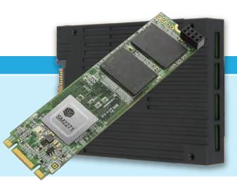
The SM2271 is a high-performance, 8-channel enterprise SATA controller enabling up to 16TB SSDs with the latest 3D TLC and QLC Flash technology. It fully maximizes the SATA interface supporting 540 MB/s Sequential Reads and 520 MB/s Sequential Writes. Accelerating time to market for lower cost SSDs, the solution includes both ASIC and turnkey firmware.
