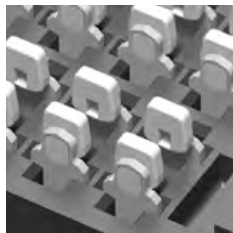
Solder charge terminations (IPC-A-610F & IPC J-STD-001F Class 3)
