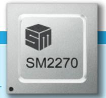
The SM2270 SSD controller enables high performance and high capacity SSD solutions with comprehensive firmware. It offers a combination of high performance, high reliability, and flexible turnkey standard NVMe and Open Channel SSD firmware ideal for use in data center applications.
