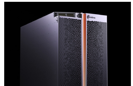
The Cerebras CS-1 server is the first available system featuring the Cerebras Wafer Scale Engine (WSE) processor which is the largest chip ever built.
