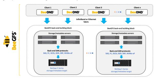
Figure 1) BeeGFS basic building block on E-Series systems.
