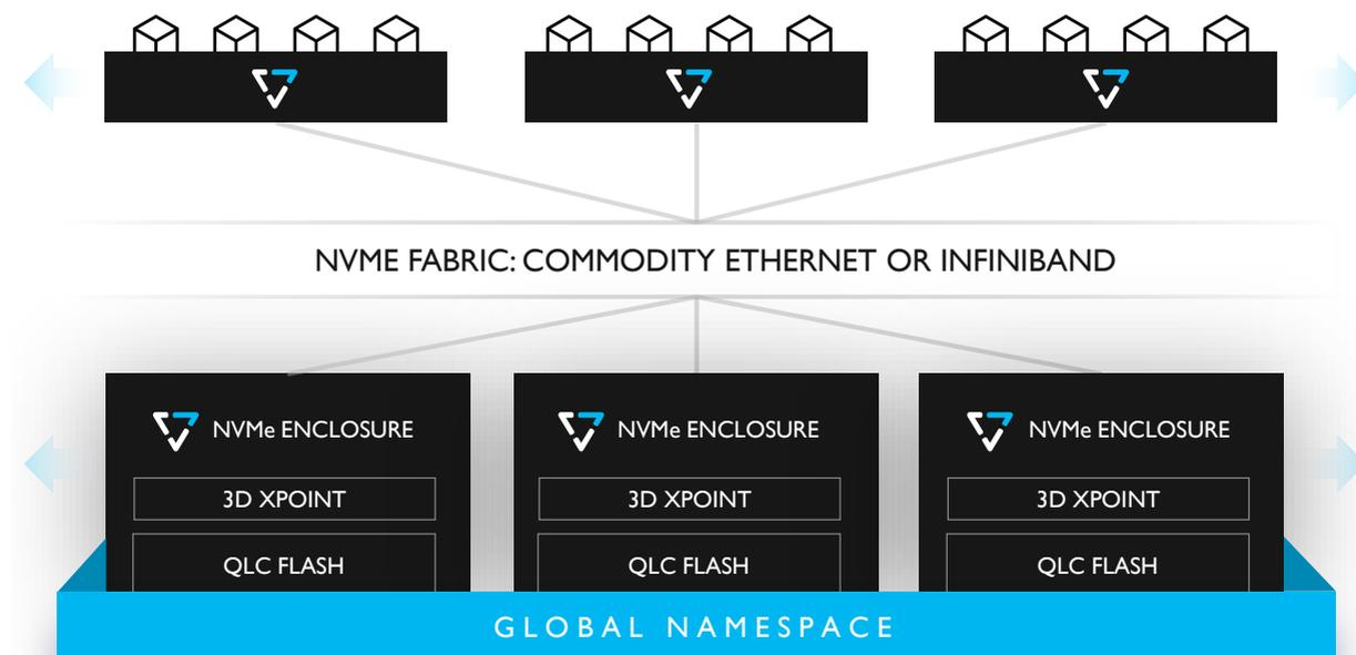
Stateless containers power VAST's system, these high-availability processes serve file and object protocols from the multi-protocol namespace. The global, shared-everything, view of the NVMe media allows VAST containers to scale massively and execute new global algorithms that enhance the efficiency of the cluster and make flash affordable for all data.
