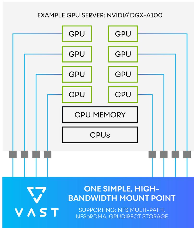
Most enterprise storage systems adhere to the standard NFS/TCP model that has been the core offering of scale-out NAS providers for decades. New AI machines need more than the 2GB/s of read throughput that a standard TCP NFS client can provide. This single-stream, non-RDMA limitation is why organizations abandon NFS in favor of parallel file systems and chose performance over simplicity.
