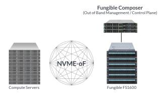
The Fungible Composer operates on a control plane that is distinct from the FS1600s' storage data plane. It runs on a 3-node self-contained quorum-based cluster for scalability and high availability. Such separation of control and data plane allows for linear scalability in capacity and performance on FSC.
