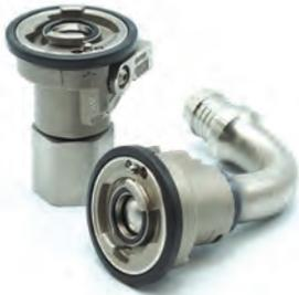
Eaton's FD83 is designed for electronics cooling applications where full flow, fluid compatibility and safety are essential. The FD83 identical halves include two interlock features to eliminate spills and ensure maximum safety. Valves cannot be opened until the coupling halves are mated and coupling halves cannot be disconnected until both halves are closed.
