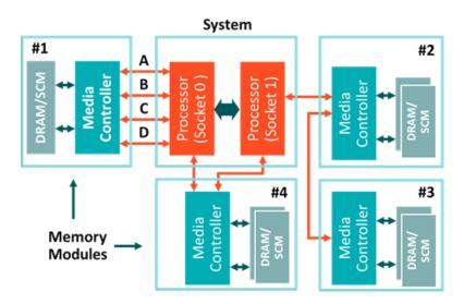
Figure 5: Gen-Z Enables Memory Subsystem Design Flexibility
