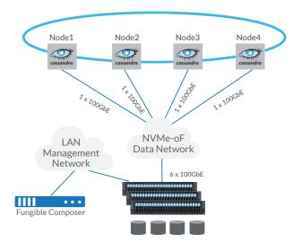
Figure 2. Apache Cassandra Deployment Using Fungible Storage Cluster Disaggregated Storage The Fungible Storage Cluster (FSC) offers unprecedented storage performance and density that allows customers to deploy large-scale disaggregated flash storage for Cassandra DB. Consequently, data center administrators can now utilize logically shared storage to replace direct attached storage for cloud-level Cassandra environments.
