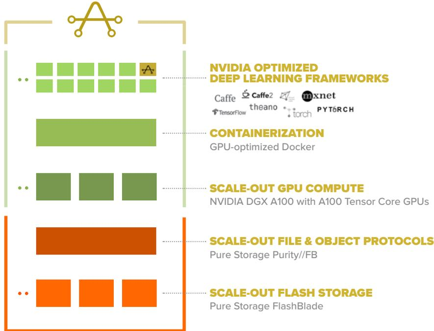
AIRI is built with a **complete software stack** enabling data scientists to get up and running in a few hours, not weeks or months.
