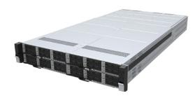
Thor is an industry-leading, high performance dense server, optimized for hyperconverged and traditional server applications. Thor incorporates Intel Xeon® and 2nd Generation Intel Xeon Scalable Processors with the support for pure NVMe and the flexibility to mix different storage technologies. This unique feature set enables unparalleled performance and flexibility for the next generation of hyperconverged and traditional server applications.
