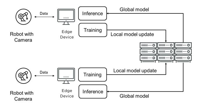
In this example, each "Robot with Camera" is taking pictures for an AI/ML application to make a prediction. The prediction is done on the Lenovo ThinkStation P330 Tiny Workstation, the edge device in this example. The edge device stores the picture and will use new data to update the model.
