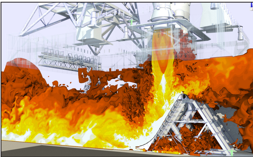
Image from a simulation of launch ignition for NASA's next-generation Space Launch System. Colors indicate temperature, where white is hotter and brown is cooler. The plume is contoured based on the air-mass fraction (that is, the fraction by mass of air vs. gas plume species). This simulation, run on the Pleiades and Electra supercomputers at the NASA Advanced Supercomputing (NAS) facility, generated hundreds of terabytes of data for each calculation. Data analysis and visualization were conducted by NAS visualization experts using custom in-house software and high-performance systems. Michael Barad, Tim Sandstrom, NASA/Ames
